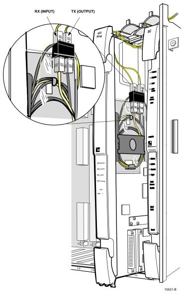
Figure 701-6. Fiber Connections on a Cellworx 622 RIC Card
